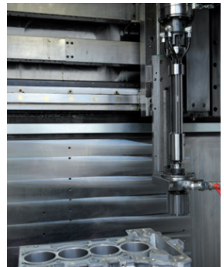
Honing unit in a PT-module
