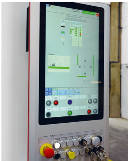
Modern Gehring operator panel with multitouch functions
