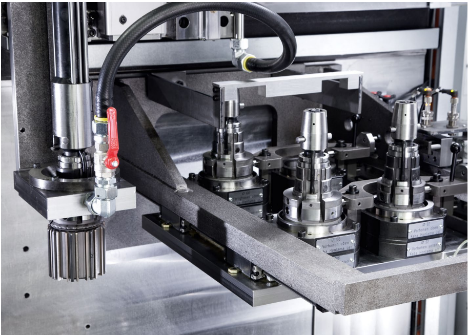
Tool changing system in a PT-module
