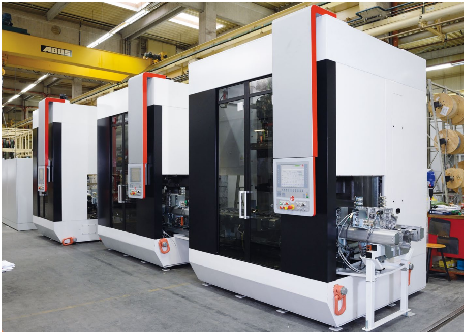
PT-module connected via Gehring conveyor
