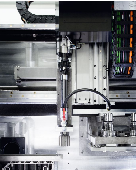
Honing unit in a PT-module
