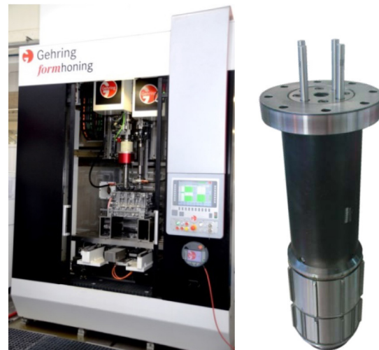
Figure 5. Honing machine for form honing and finishing, form honing tool
