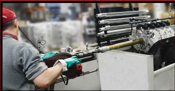
A Sunnen CH-100 fixtures a block for manual honing of cam tunnel.
