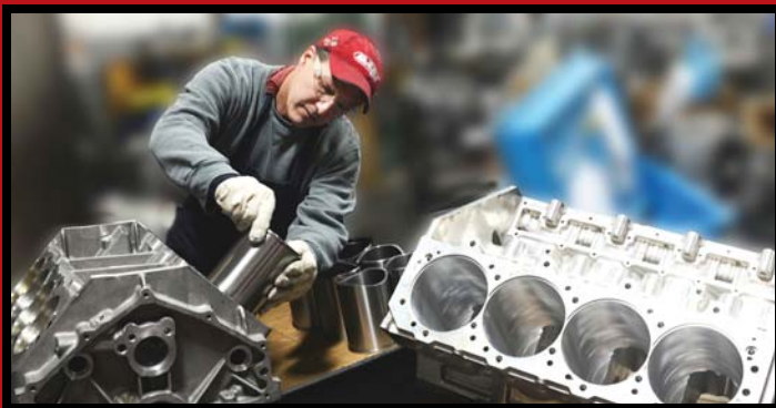
Technician Bob Dimitrijevič installs Darton iron sleeves in cast aluminum block, while a billet aluminum racing block awaits installation. Aluminum block bores are honed for size and geometry before liner installation.
