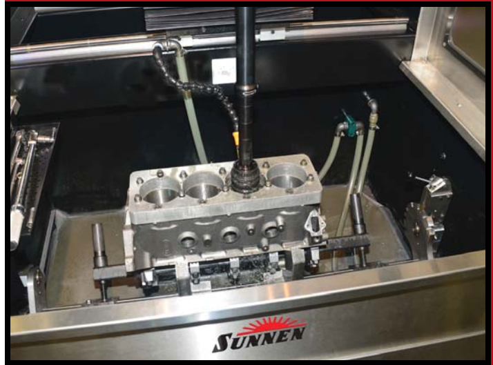
A small block Chevrolet performance block being honed in the new SV-20 machine.
