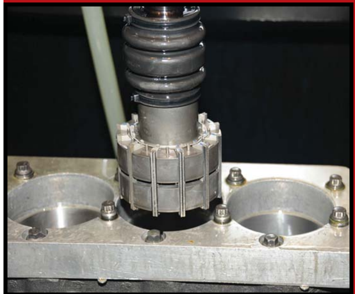
Sunnen's two-stage diamond abrasive honing tool does roughing and finishing with 220- and 500-grit abrasive without pause for stone change. The advanced control system on the SV-20 allows Dart to achieve a wide range of finishes with these two abrasives.
