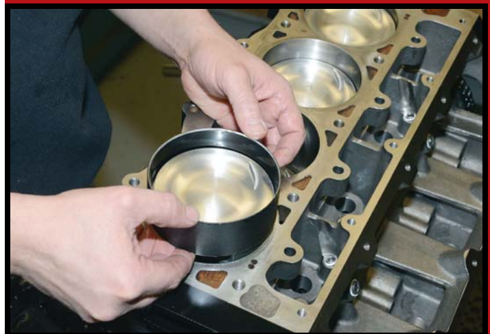
A ring compressor eliminates pre-compression of the rings and a square installation in the bore.
