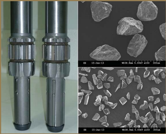
Diagram 4: Hone Tools with Lower Guides and CBN-Abrasive Crystals (B213 / B46)
